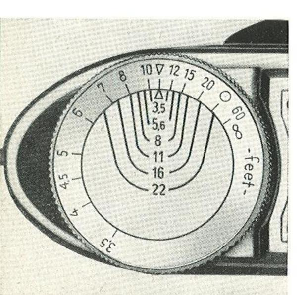
The unobserved snapshot leads often to a surprisingly nice picture. One foregoes the use of the rangefinder and sets ring 13 to the near-point  $\nabla$  for subjects between 8 ft and 16 ft and to the distant-point O for subjects between 16 ft and  $\infty$  (infinity). The camera remains closed. The aperture is set to f 11 — best well in advance.
