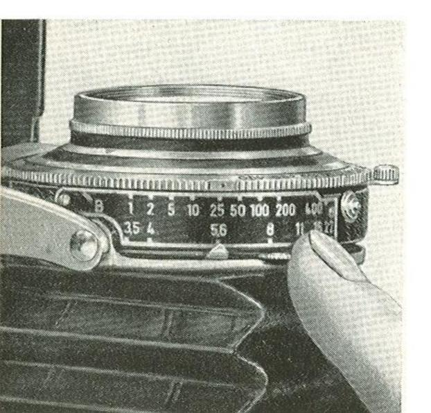
The aperture controls the amount of light reaching the film, and further influences the depth of focus (see page 17). It is set by the lever 4. The indicator to the left of the aperture lever has to show to the aperture required.
