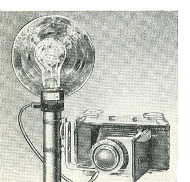
The internally synchronised shutter allows the use of the usual flash bulbs and speed lamps, with the help of which instantaneous photographs in poor light and complete darkness may be taken. The flash unit has to be connected by cable to the flash contact 8. After setting and on releasing, shutter and flash are released simultaneously at the moment the shutter is fully opened up (O-synchronisation).
