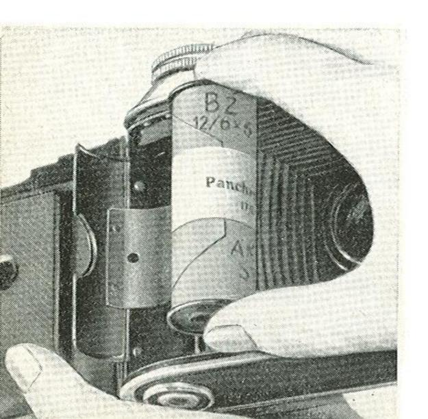
To the right and left of the large film aperture in the camera, are the two spool chambers. Into the left one (below the range-finder knob) goes the unexposed film, while the right one carries the empty take-up spool (see also page 16).
