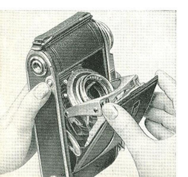
Take the camera into your left hand, and press the button on the left side of the camera body with the thumb. The baseboard will open up and has to be pulled down with two fingers of the right hand, on either edge until it engages with an audible "click".
