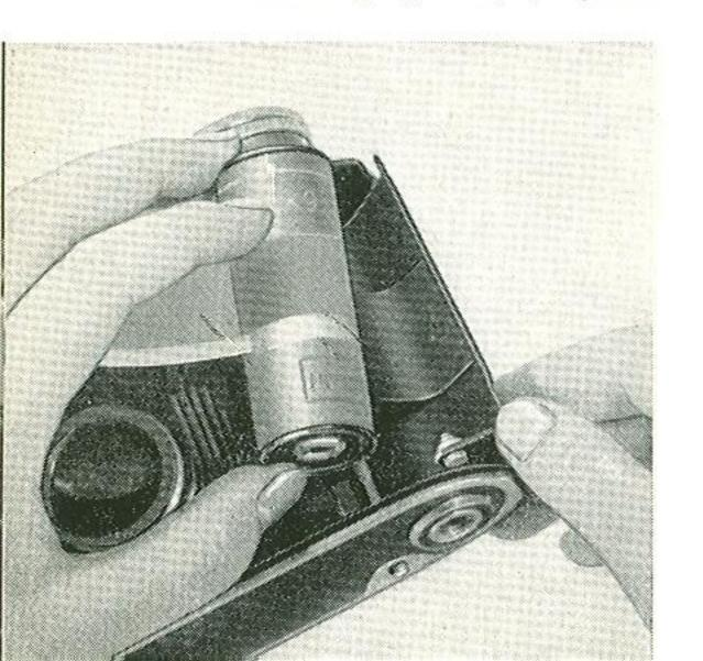
After the eighth exposure the film key is turned until the end of the backing paper has passed the film window. Open camera back, pull out film key and lock by slightly turning it. Swing out spool holder, remove film (hold it tightly so that it does not unwind) fold up backing paper and seal it with the gummed paper. The film should be removed in subdued daylight.
